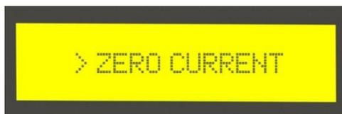
→ To make the current zero, hold the fault reset button for 3 seconds and the LCD will display the following message.
